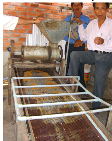
Husk grinding machine after pepper being soaked
